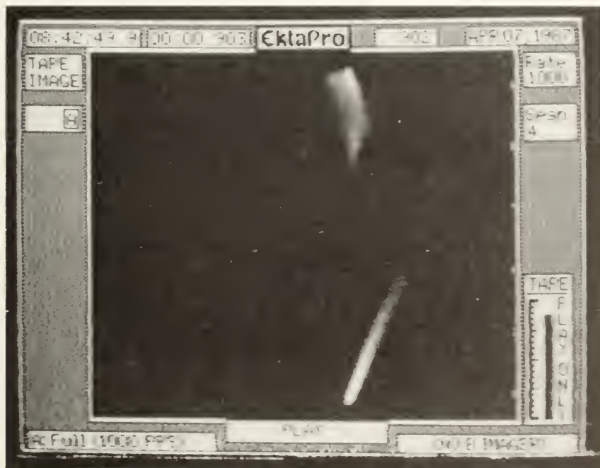
Figure 29—A well-formed typical arc; b,c,d: fast video of the shut-off of the same arc.
